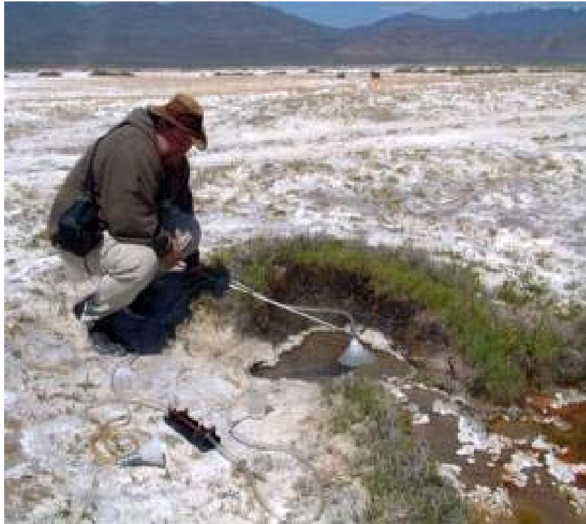
Arizona State geochemist Matthijs van Soest samples surface water in the northern Basin and Range. The sample is collected without direct exposure to air and stored in the copper tube, foreground left, which will be sealed by crimping. (Credit: Image courtesy of DOE/Lawrence Berkeley National Laboratory)
